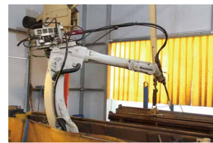
Automatic Welding Robot
